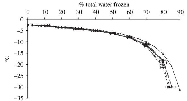
**Figure 2** Theoretical (no symbols) and experimental freezing curves for ice cream mixes with 15% sucrose (◇), 12% sucrose/3% trehalose (Δ), 9% sucrose/6% trehalose (◊), 6% sucrose/9% trehalose (\*), 3% sucrose/12% trehalose (×) and 15% trehalose (–).
