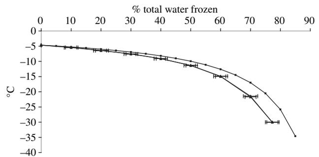
**Figure 3** Theoretical (no symbols) and experimental freezing curves for 40% trehalose (Δ) and 40% sucrose (×) solutions.
